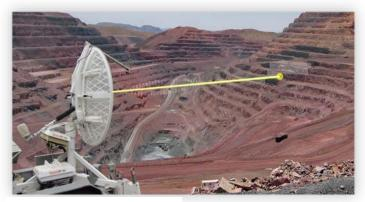
Radar-based monitoring solution
