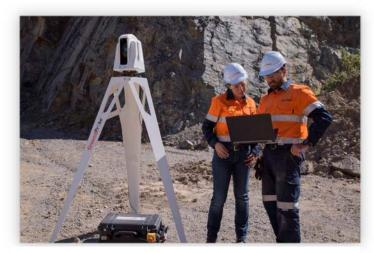
Geotech Monitoring Station (GMS) - laser-based monitoring solution
