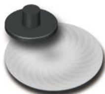
Back grinding (wafer thinning)
