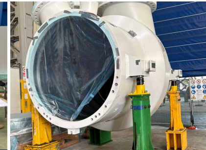
Compressor casing for Mixed Refrigerant Compressors (Baker Hughes)
