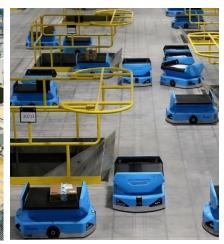
Single piece picking, robotics integration to automate picking and sorting functions
