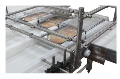
Custom designed sanitary and easy to clean conveyors engineered to the strictest USDA guidelines
