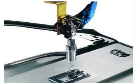
Cold Material Dispensing
