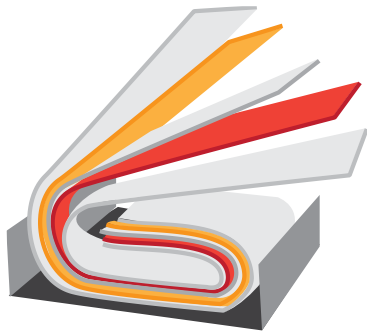
Conventional Wound Lithium-ion Cell
