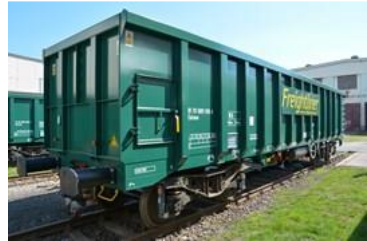
Converted Freightliner coal wagon for aggregate
