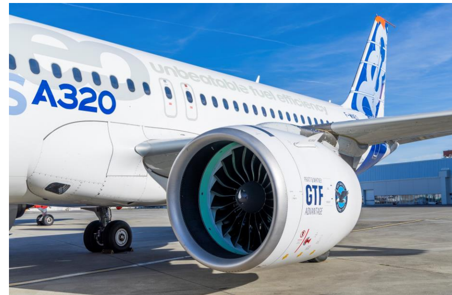
The Pratt & Whitney GTF Advantage™ engine, seen here in Toulouse, France, started development flight testing for the A320neo family. The engine has completed more than 2,400 hours and 7,800 cycles of testing, including a successful test on 100% sustainable aviation fuel (SAF). Engine certification will continue through the first half of 2023.
