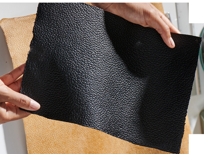
A sustainable leather-like material called Mylo™, engineered from mycelium, a fungus that grows naturally Photo courtesy of Bolt Threads
