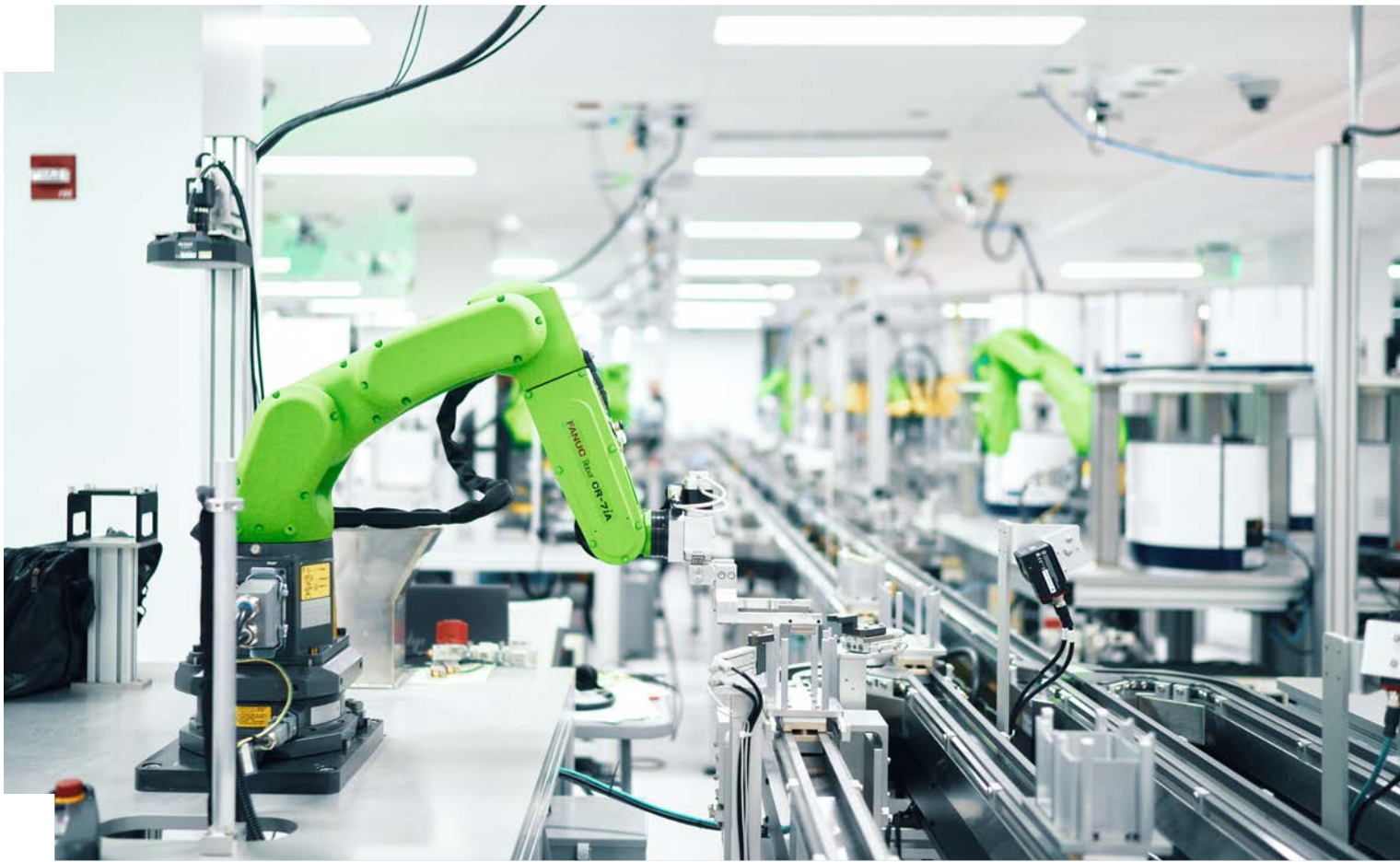
Liquid handling robots used to automate high-throughput screening of biological samples Photo courtesy of Ginkgo Bioworks
