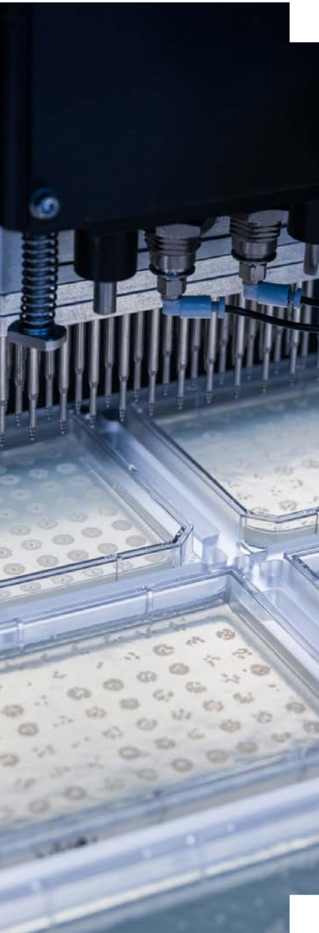
A colony picker, used to identify new bacterial strains that can create new products Photo courtesy of Ginkgo Bioworks
