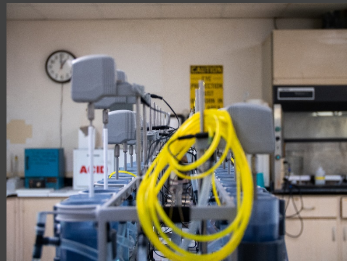
48-stage lab-scale solvent extraction (SX) REE separation occurring today at Energy Fuels' White Mesa Mill
